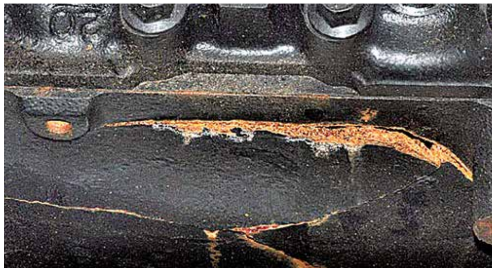
Water expands when it freezes and not properly winterizing your engine can lead to a cracked block, necessitating engine replacement.
