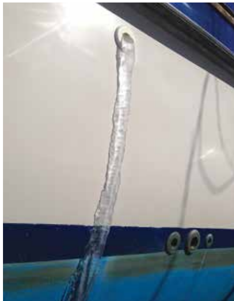
Frozen meltwater can damage thru-hull fittings.
