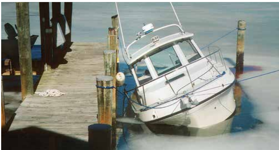
Boats stored in water over winter are vulnerable to sinking damage if a hose or thru-hull fails.
