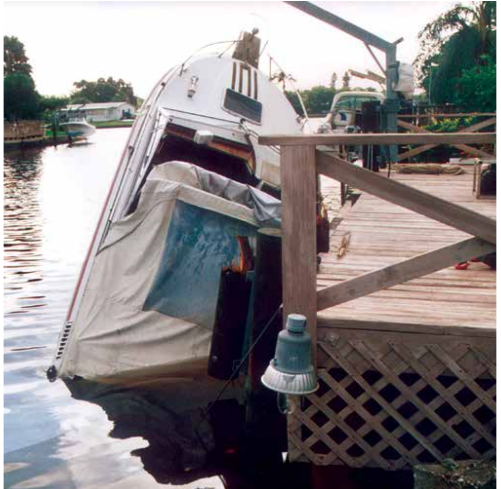
Rain or snow can make a boat too heavy for its lift.
