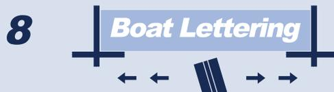
8. When the graphics are in position, squeegee the graphic (make sure you press firmly with the squeegee to push out any air bubbles and the soap and water solution).
