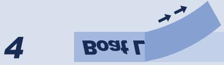
4. Carefully pull backing paper away from transfer tape. It is important that there is no wind blowing during this process.
