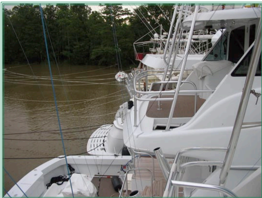
Using multiple anchors and lines ashore greatly increases the chances boats will survive in a hurricane hole.
