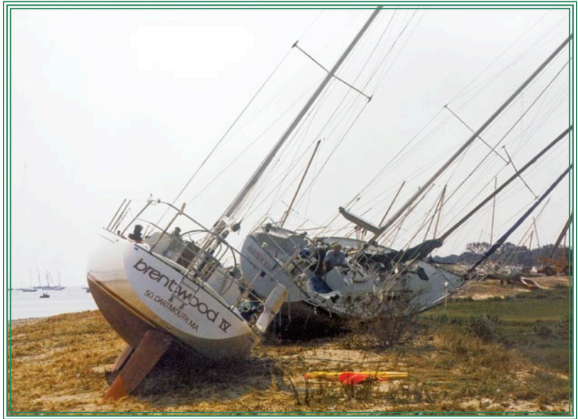
Hundreds of moorings were pulled out when Hurricanes Bob and Gloria swept through New England. Probably an equal number failed because of chafe.
