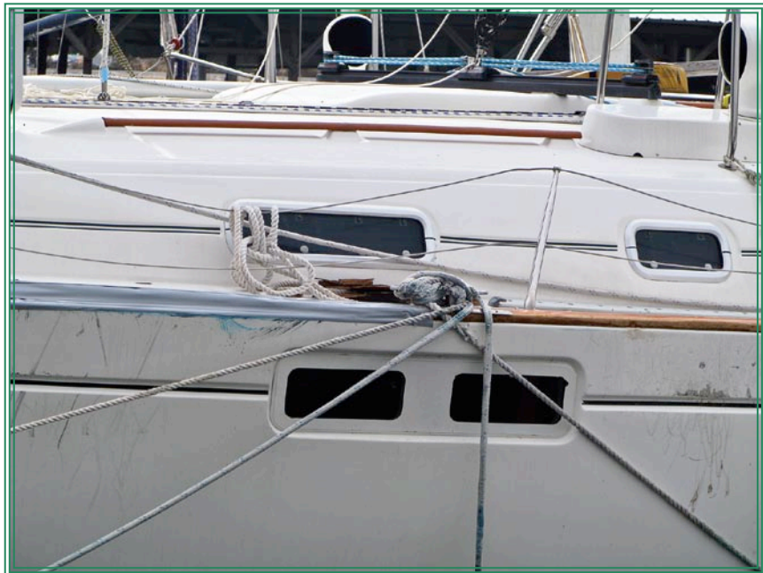
Using more and longer lines often pays off. This was one of the boats at the Houston Yacht Club that survived Ike.
