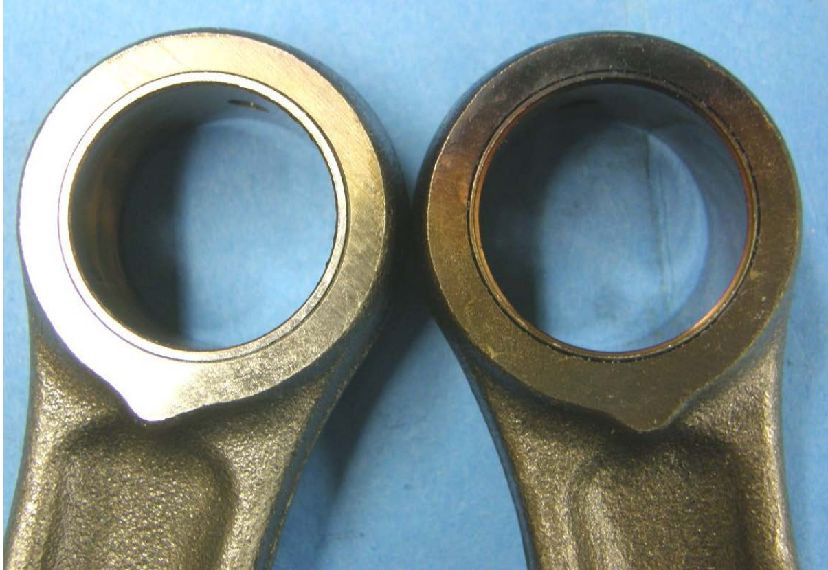
Figure 42: Connecting Rod Carbon Deposit Comparison, Cylinder 2, E0 on Left, E15 on Right
